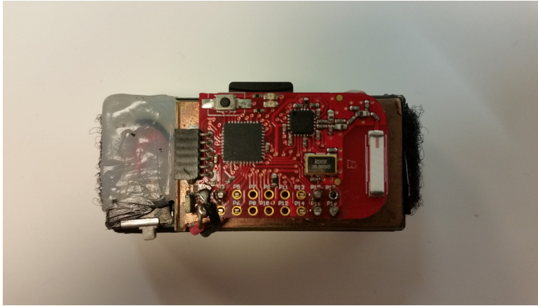
Fig. 7: Wearable radio transceiver. The device is approximately 50 mm x 20 mm x 20 mm.
