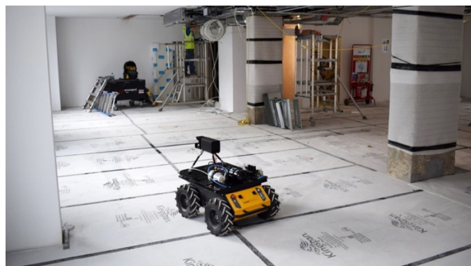
Figur 11: Robotskanner fra Scaled Robotics. (Aga 2018)
