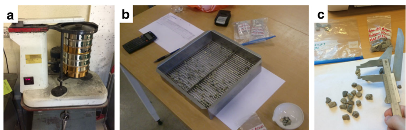
Fig. 3 Performing (a) particle size distribution with multiple sieves on dry material, (b) the flakiness index test with a grid sieve, and (c) the shape index test with a customised particle slide gauge
