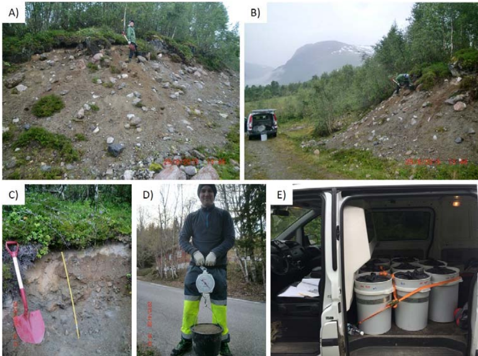
Figure 3.2 (A & B) show a typical till sampling site (sample no. 14, province D) in a non-vegetated slope cut reachable by car, while (C) shows the excavation of the sample pit (the carpenter's ruler is 1 m). (D) Shows the use of a spring scale to collect the recommended amount of material per sample, i.e., minimum 53 kg. (E) Shows how the samples were transported by car in individual, sealed plastic 50 litres barrels, i.e., one sample per barrel. See also appendix 1 and 2 for coordinates and photographs of each sample site. (B & C) are from Opsal (2017).
