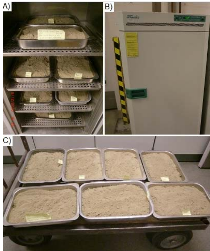
Figure 3.6 The process of drying till samples before shear testing. (A) Approx. 40 kg of material from each sample was dried in shallow pans in (B) a drying oven at 110\text{ }^{\circ}\text{C} \pm 5\text{ }^{\circ}\text{C} for a minimum of 16 hours. (C) A dried sample ready for shear testing.
