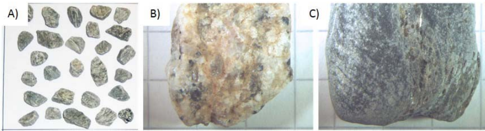
Figure 3.16 (A) An example of a sieved fraction (material retained on the 10-mm sieve) of sample material (sample no. 11, prov. D) used together with other fractions for an evaluation of the most common particle roundness category of the till sample. (B & C) show examples of surface texture differences between particles (10-mm fraction) categorised as ‘rough’ (no. 9, prov. C) and ‘smooth’ (no. 21, prov. E), respectively (the paper squares behind the particles are 5 x 5 mm). From Opsal & Langeland (2018).
