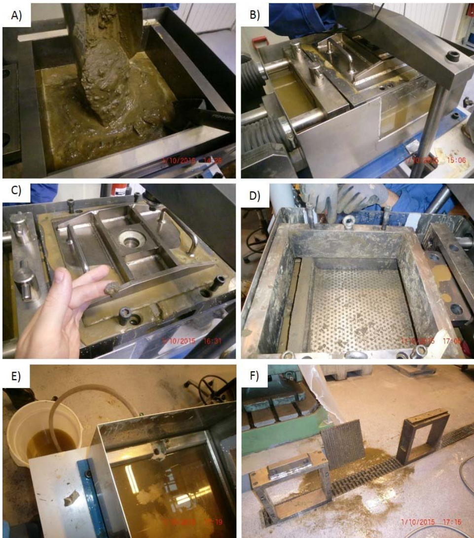
Figure 3.8 (A–C) show parts of the difficult and rather messy process of shear testing a till sample (from site no. 23, prov. E) in a fully saturated condition. (D–F) show the process of cleaning the apparatus after the shear test has been aborted. As can be seen, especially from the figures (D–F), significant amounts of material (particularly fines) are lost in suspension when shear testing and cleaning.
