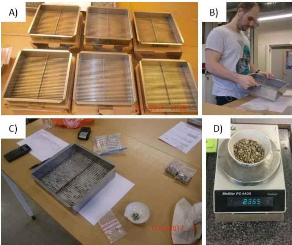
Figure 3.14 (A) The flakiness index test by using a total of six grid sieves. (B & C) Performing manual sieving. (D) Afterward, the material portions were weighed to calculate the FI value of the till sample. (C) is from Opsal & Langeland (2018).
