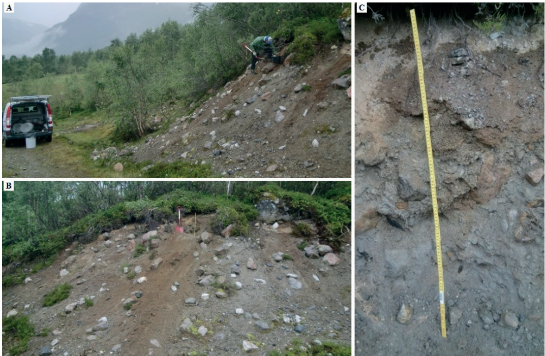
Figure 2. An example of a typical till sampling location, here from sample no. 14, Jordalen in Voss municipality, Hordaland county: (A) A non-vegetated slope cut reachable by car, (B) Overview of the sample site (pit marked by shovel and carpenter's ruler), (C) Excavation of sample pit (the carpenter's ruler is 1 m).
