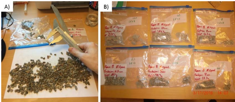
Figure 3.15 (A) The shape index test by using a customised particle slide gauge to determine the length and thickness of particles. (B) After a completed shape index test, the elongated particles were placed in the blue plastic bags, while the cubical particles were placed in the smaller red bags. The portions of material were thereafter weighed to calculate the SI value of the till sample.
