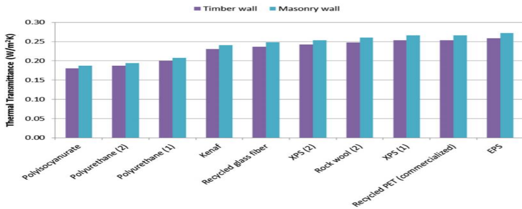
Figure 10 The thermal transmittance of the case study.
