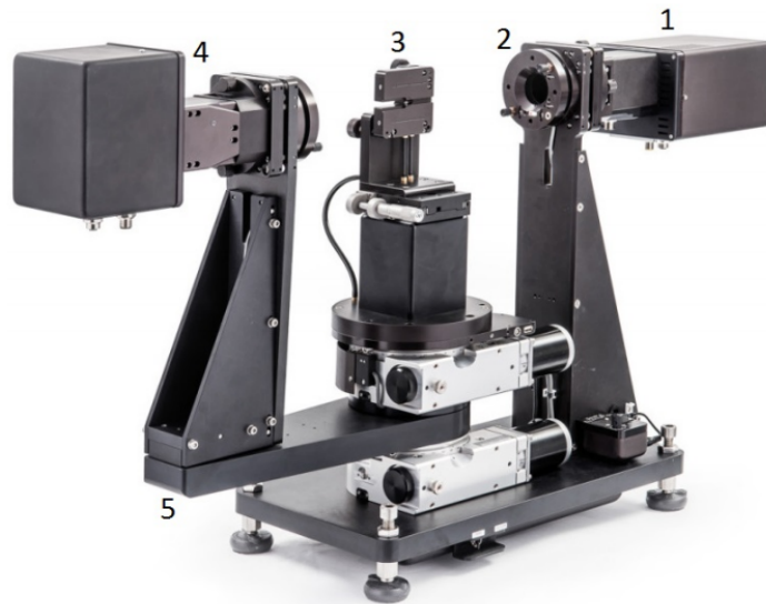
Figure 3.2: Experimental setup of the RC2 ellipsometer with 1) light source, 2) source optics, 3) vertical sample mount, 4) receiver optics and 5) goniometer arm for variable angle measurements. Figure taken from [6], originally adapted from [31].
