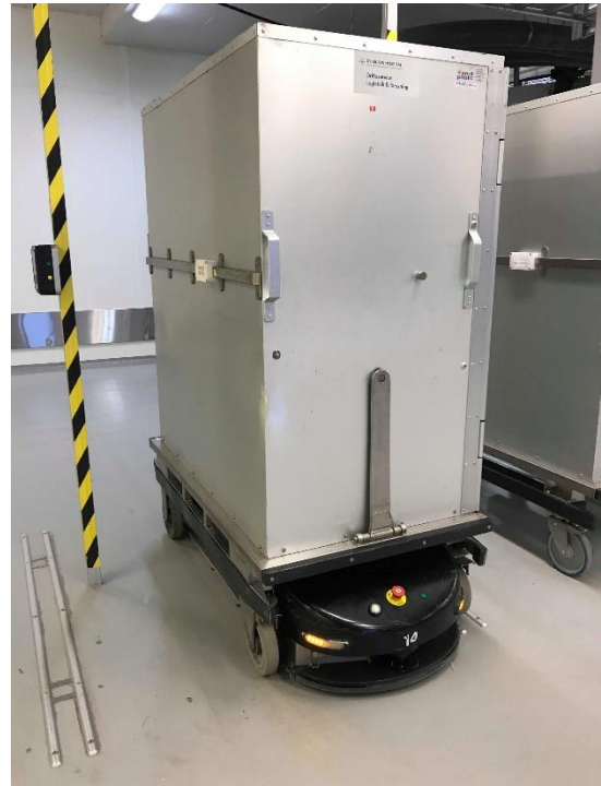
Figure 14: A Warehouse container picked up by an AGV at a pickup station.
