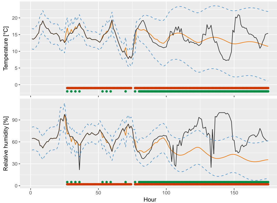
Figure 6.3: Predicted temperature and relative humidity plotted in orange with a 95% prediction interval presented in dotted blue lines. The black line is the real data collected from the solar panel. The red and green circles represent the decisions presented in Figure 6.1 and Table 6.1.
