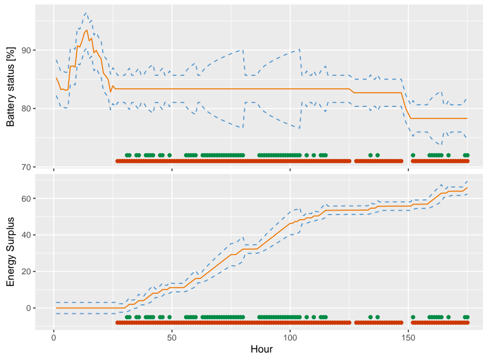
Figure 6.13: Behaviour of the battery when threshold (6.2) and (6.4) are used as activation threshold. Orange line in the upper plot is assumed battery status while lower plot is the development of accumulated energy surplus. Dotted blue lines are 95% prediction interval computed from the variance of the temperature. The red and green circles represent the decisions presented in Figure 6.1 and Table 6.1.
