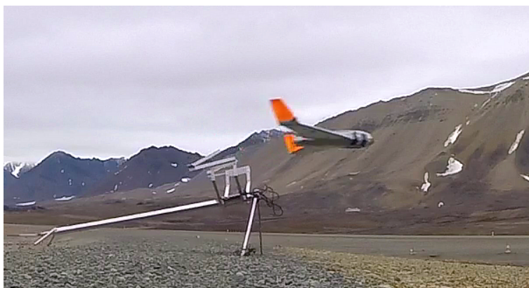
Figure 3.8: Launch of X8 using a catapult.
