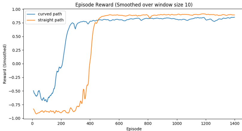
Figure 26: The training reward of the Mariner model with 10 [s] time step on the curved and the straight path.
