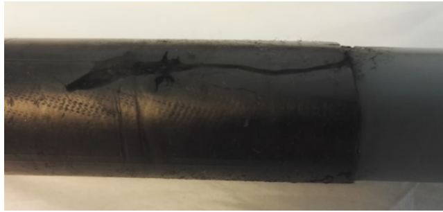
Figure 53: Tracking observed on the outer semiconductor.
