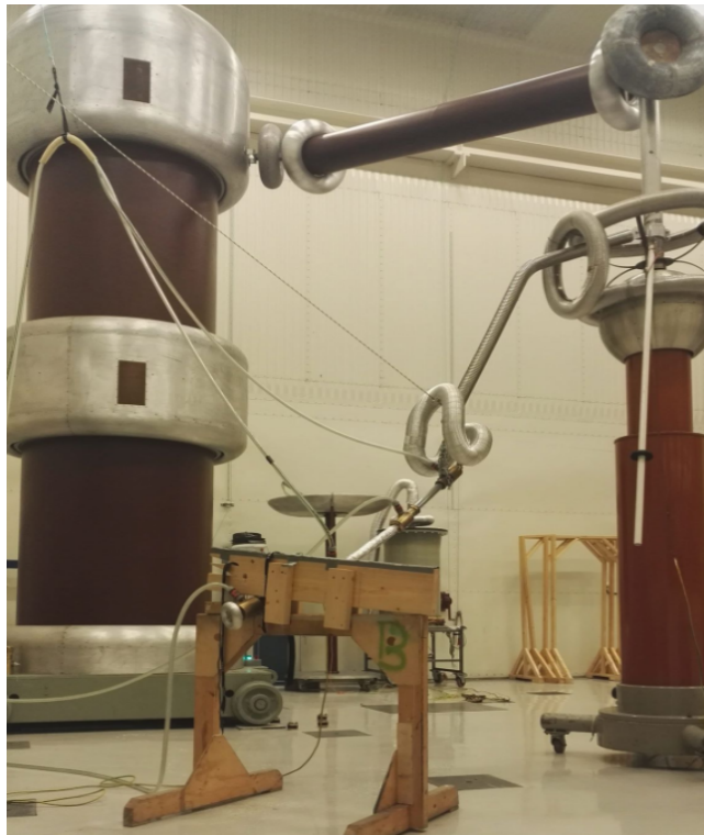
Figure 35: Picture of the setup used to measure the test objects' break-down voltages. The transformer can be seen on the left, and the coupling capacitor is on the right. The test object with water terminations can be seen in the middle.
