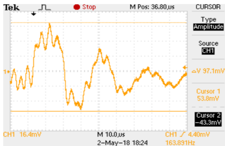
Figure 41: The view of the oscilloscope as PD is found in a measuring point. As can be seen in the figure, cursors are used to measure the peak-to-peak magnitude of the signal.
