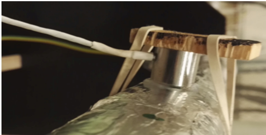
Figure 33: Picture of how the acoustic sensor is fastened to the test object, by help of a piece of wood and an elastic band. Vaseline ensures good contact between the test object and sensor.
