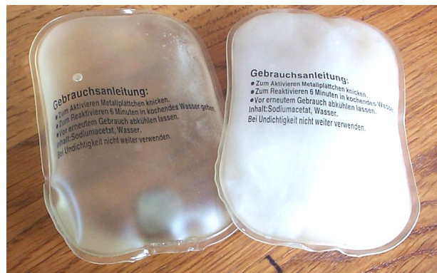
Figure 1.15: Image of melted and solidified hand warmers with PCM (Pawar, n.d.)
