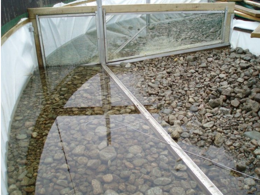
Fig. A7: Inside of the arena: Detail of the downward slope from the shallow to the deep area. The metal rail in the middle will hold the trap door in place once lowered. Fine plastic mesh is fastened to a wooden construction separating the sections from each other.
