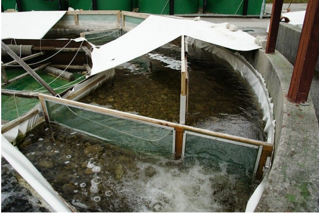
Fig. A5: One of the arenas during the 20 hours acclimatization period seen from upstream. White tarps cover about 50% of each section. The "trap doors" are locked in place above the water surface and are ready to get dropped by removing the metal bolts that are attached to ropes.
