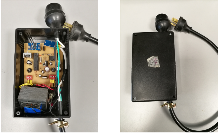
Figure 6.1: The La Salle Wi-Fi sensor developed by Lara in [24] to measure current of household appliances.
