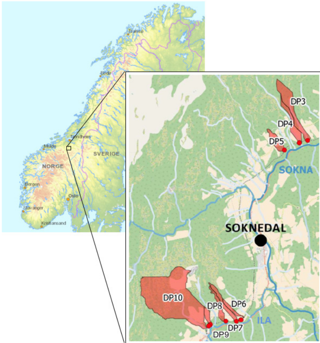
Figure 3.5 Location and catchments to culverts/damage points where Dovrebanen is marked with a dotted line - from Use of a parsimonious rainfall-runoff model for flood peak modelling in small ungauged catchments in Norway (Vauclin, 2017).
