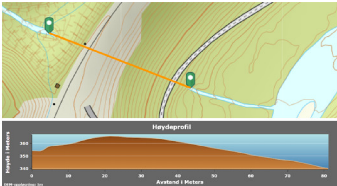
Figure 3.6 Height profile for culvert DP10 created in Høydedata to estimate length and slope.
