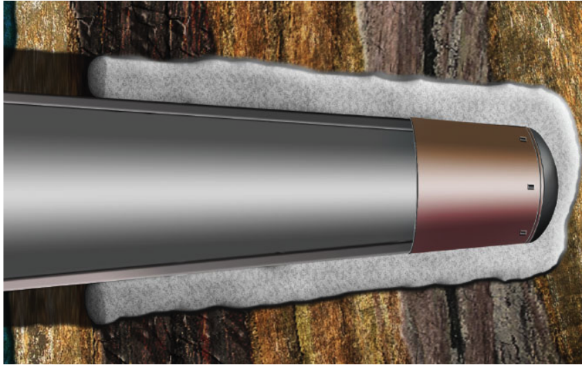
Figure 2.4.: An illustration of cement flow in the annulus through the various formations [3].
