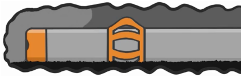
Figure 1.2.: Inadequate cementing due to the presence of cuttings in the wellbore (Courtesy of Centraflow).
