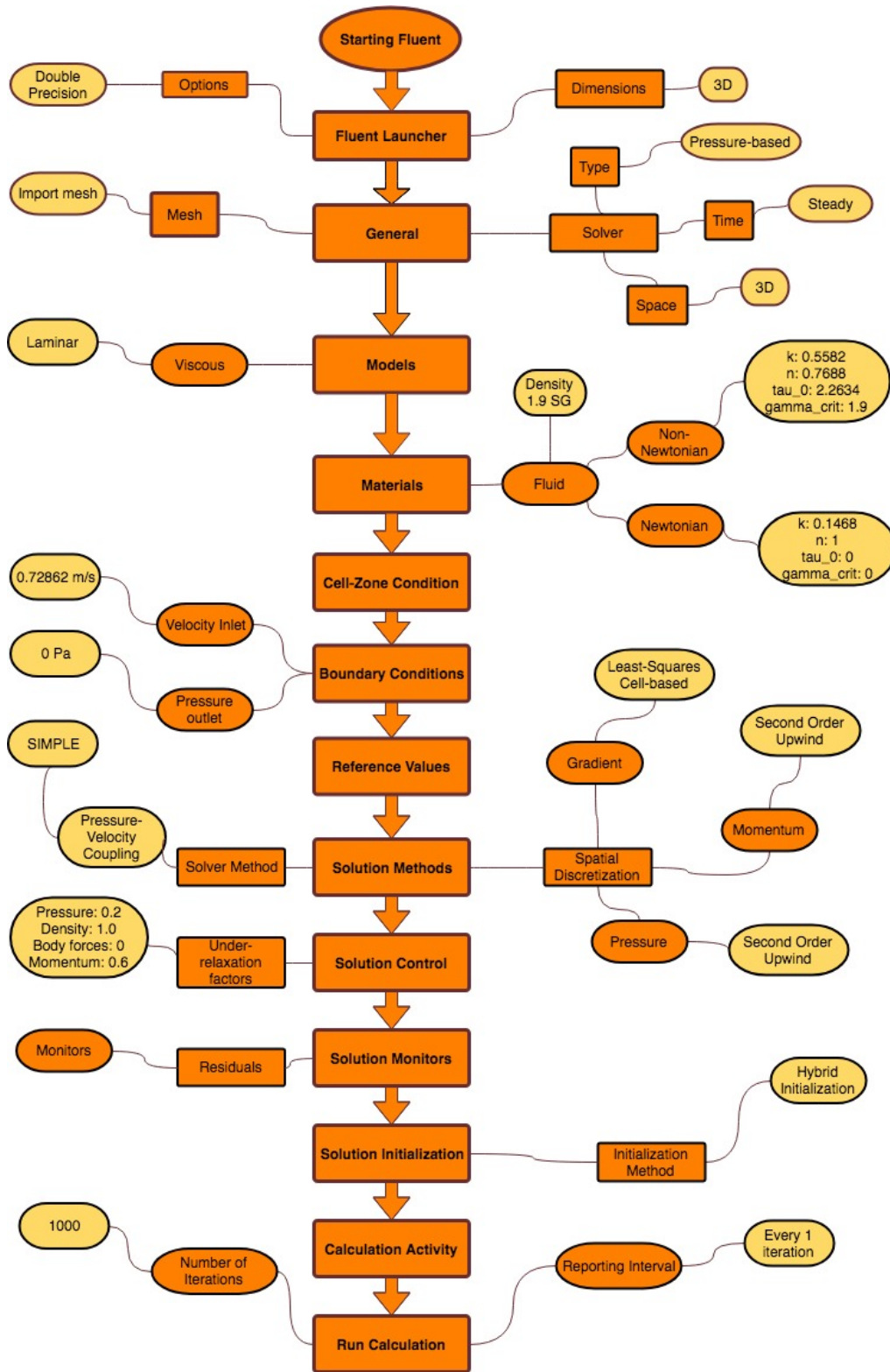
Figure 6.10.: Schematic of CFD set-up in Fluent for performing single-phase simulations.
