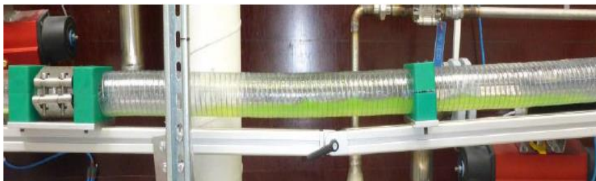
Figure2.26(b): Liquid accumulation at the dip [3, p.35].
