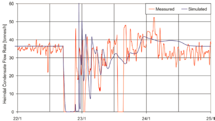
Figure 2.10: Measured and simulated condensate rate at Heimdal [11, p.9].
