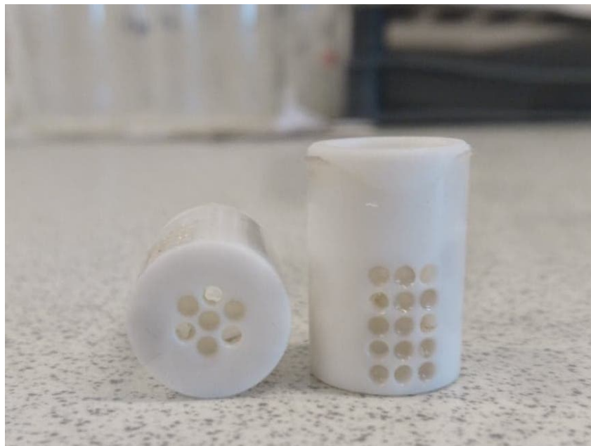
Figure 3.4: The Teflon caps coated with PDMS-TiO 2 /Ag. Some of the holes had to be reopened with a needle after coating.
