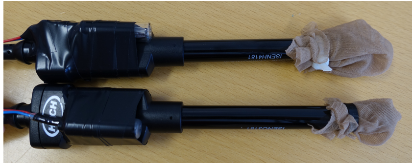
Figure 3.2: Before the second experiment in RAS where a nylon filter and vibration were used to examine the effect on biofouling.
