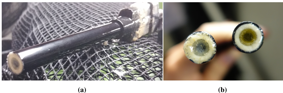
Figure 4.4: Amount of biofouling after three weeks (a) and in the end of the experiment, 5 weeks (b) in the flow through system with smolt.
