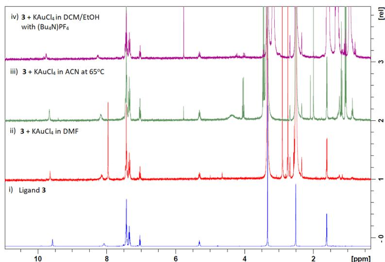
Figure 13:  $^1\text{H}$  NMR spectra of squaramide **3** (i), the coordination attempt of squaramide **3** with  $\text{KAuCl}_4$  in DMF after stirring 4 days (ii), the coordination attempt of squaramide **3** with  $\text{KAuCl}_4$  in ACN at 65 °C after stirring 3 days (iii) and the coordination attempt of squaramide **3** with  $\text{KAuCl}_4$  in DCM/EtOH with  $(\text{Bu}_4\text{N})\text{PF}_4$  after stirring 2 days.
