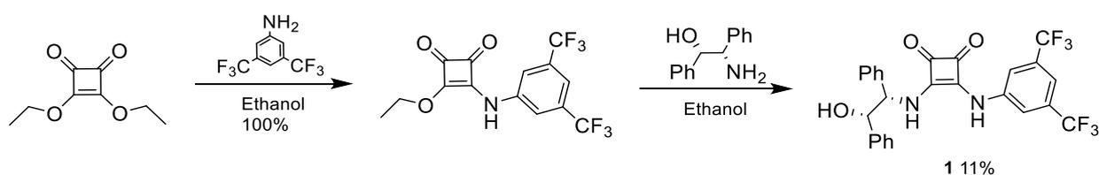
Scheme 9: Step-wise synthesis of squaramide 1 from squaric ethyl ester, 3,5-bis(trifluoromethyl) aniline and (1S,2S)-2-amino-1,2-diphenylethan-1-ol.
