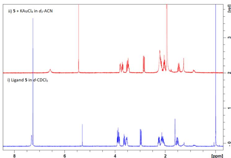
Figure 19:  $^1\text{H}$  NMR spectra of the ligand squaramide **5** (i) in  $d\text{-CDCl}_3$  and the product after an attempted coordination of the ligand with  $\text{KAuCl}_4$  in  $d_3\text{-ACN}$  (ii).
