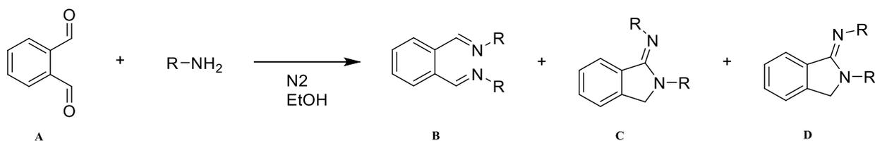
Scheme 5: Reaction between phthalaldehyde (**A**) and a primary amine yielding three different products,  $\gamma$ -diimine, (*E*)-iminoisoindoline (**C**) and (*Z*)-iminoisoindoline (**D**).
