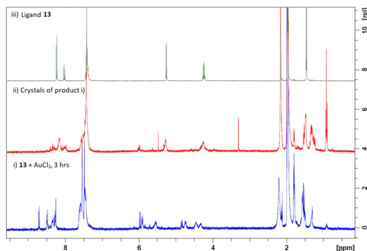
Figure 25: <sup>1</sup>H NMR spectra of the attempted formation of gold-complex **14** after three hours (i), crystals formed from the same attempt (ii) and oxazoline ligand **13** (iii).
