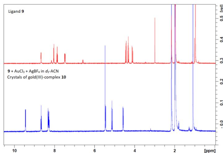
Figure 22:  $^1\text{H}$  NMR spectrum of crystals of gold(III)-complex **10** compared to the  $^1\text{H}$  NMR spectrum of ligand **9**.
