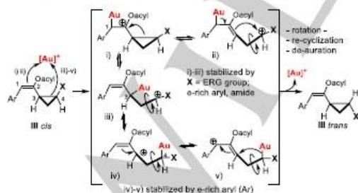
**Scheme 3.** Possible intermediates in *cis*-to-*trans* vinylcyclopropyl isomerization.
