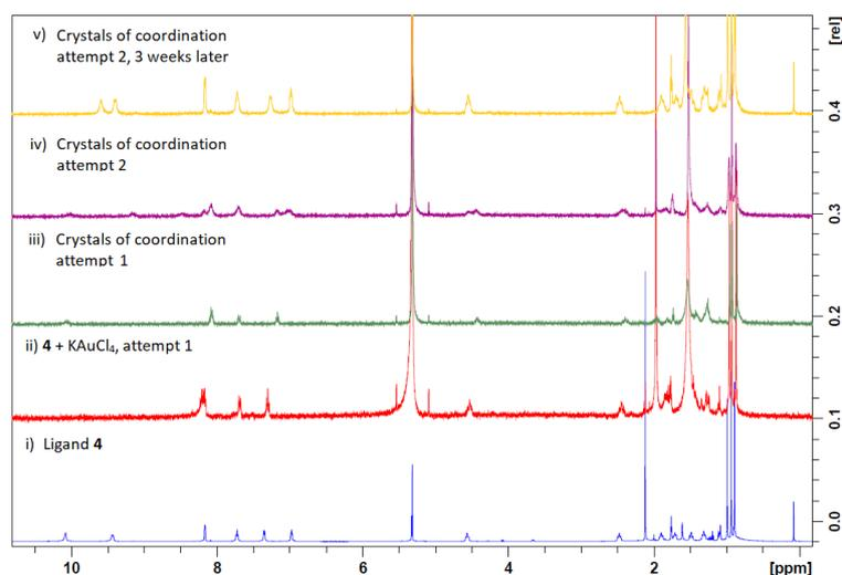
Figure 16:  $^1\text{H}$  NMR spectra of the ligand squaramide **4** (i), after the first coordination attempt of squaramide **4** with  $\text{KAuCl}_4$  (ii), crystals from the first coordination attempt (iii), crystals of the second coordination attempt (iv), and crystals of the second coordination attempt after three weeks in the freezer (v).
