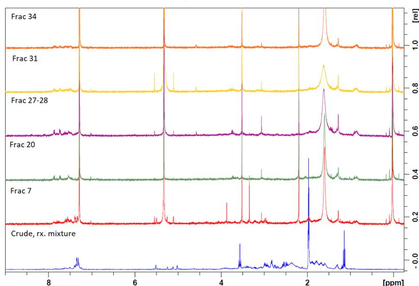
Figure 12:  $^1\text{H}$  NMR spectra from the attempted synthesis of (*E*)-*N*,2-bis(((*S*)-pyrrolidin-2-yl)methyl)isoindolin-1-imine. From the bottom and up, crude product before purification on column chromatography, and the fractions 7, 20, 27-28, 31 and 34 after purification on column chromatography.
