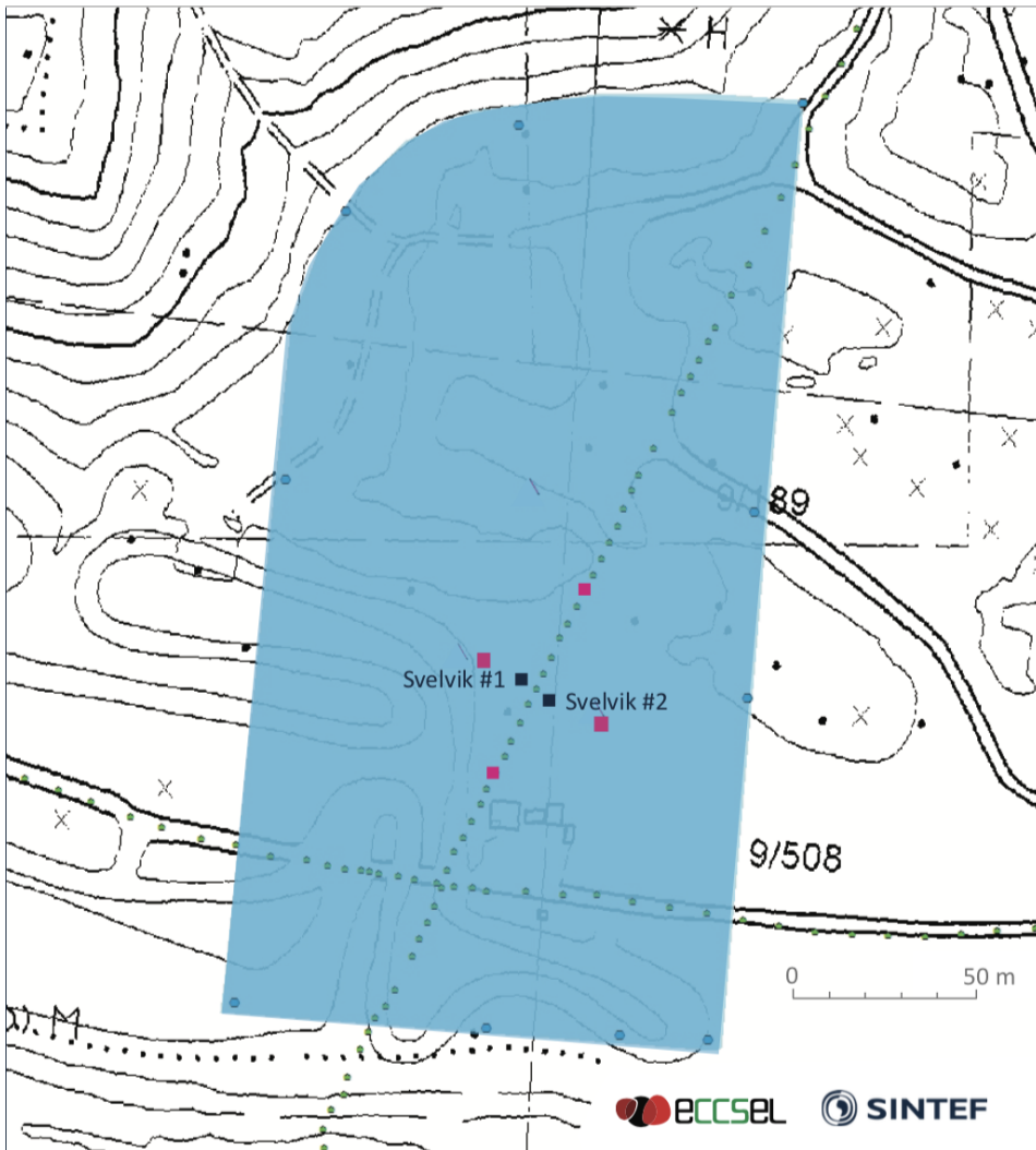
Figure 2.7: Illustration of a possible placement of the monitoring wells around the Svelvik #2 well. Monitoring wells shown as pink squares. Adapted from Ringstad (2017)
