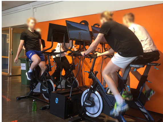
Figure 21.1: The test setup for the experiment, consisting of four exercise bikes each with a monitor attached
