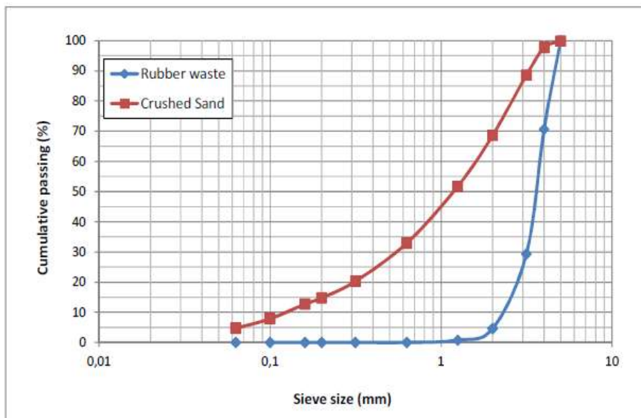
Fig. 1. Particle size distribution of used sand and rubber waste.
