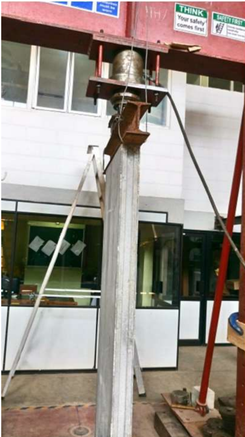
Fig. 5. Wall panel being tested for compressive strength.
