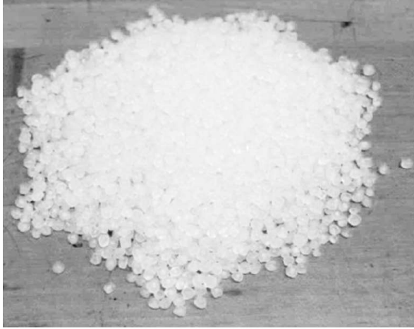
Fig. 1. Polyethylene beads used in the preparation of TI-LWC.
