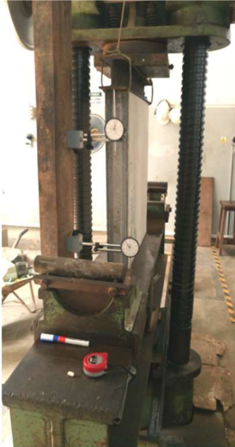
Fig. 2. A Short Wall panel being tested for compressive strength.
