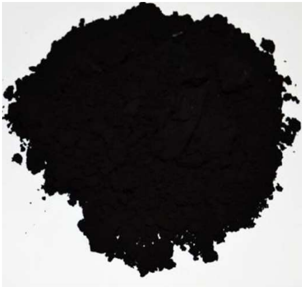
Fig. 3. Oil ash used in the preparation of TI-LWC.
