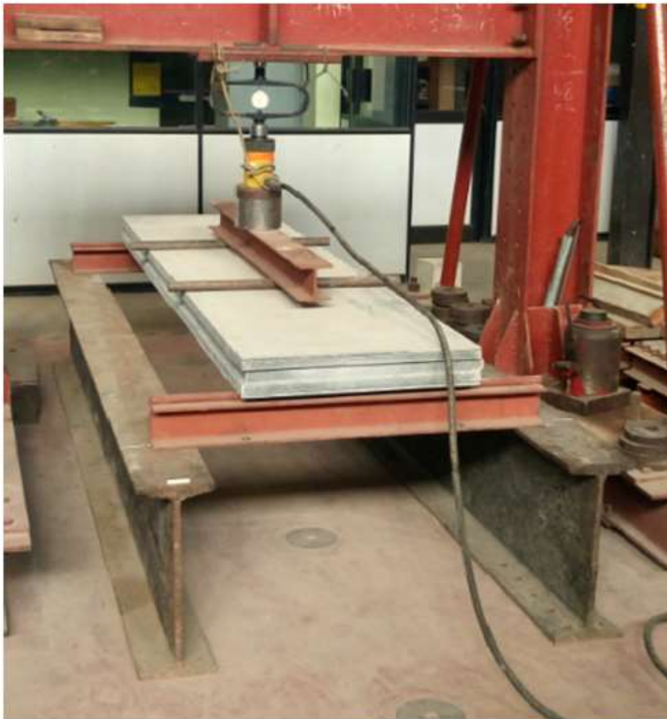
Fig. 6. Wall panel being tested for flexural strength with third point loading.
