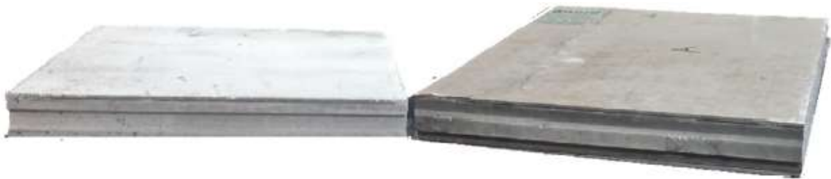
Fig. 7. The tongue and groove arrangement.
