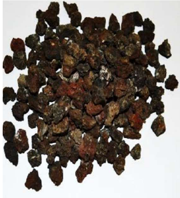
Fig. 2. Scoria aggregate used in the preparation of TI-LWC.
