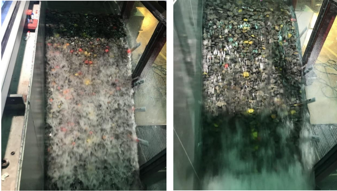
Figure 178 Two different overtopping scenarios during tests. Low discharge resulting in highly aerated flow over the entire riprap on the left and high discharge resulting in a complete clearly defined depth of water over the riprap layer on the right.
