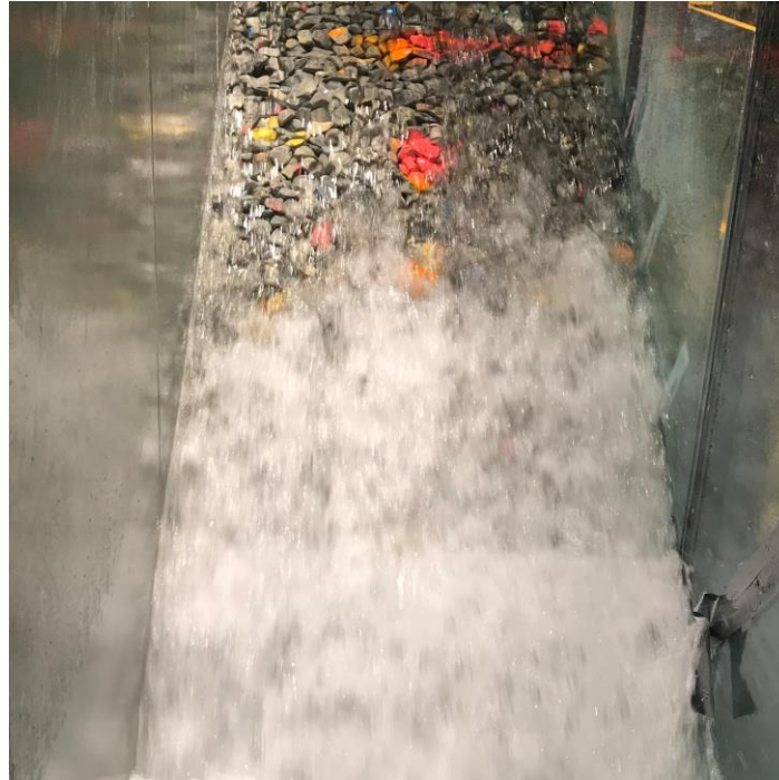
Figure 2 Laboratory model test which shows highly turbulent flow condition at the riprap toe on the downstream slope of an embankment dam. Photo by K.N. Opore
