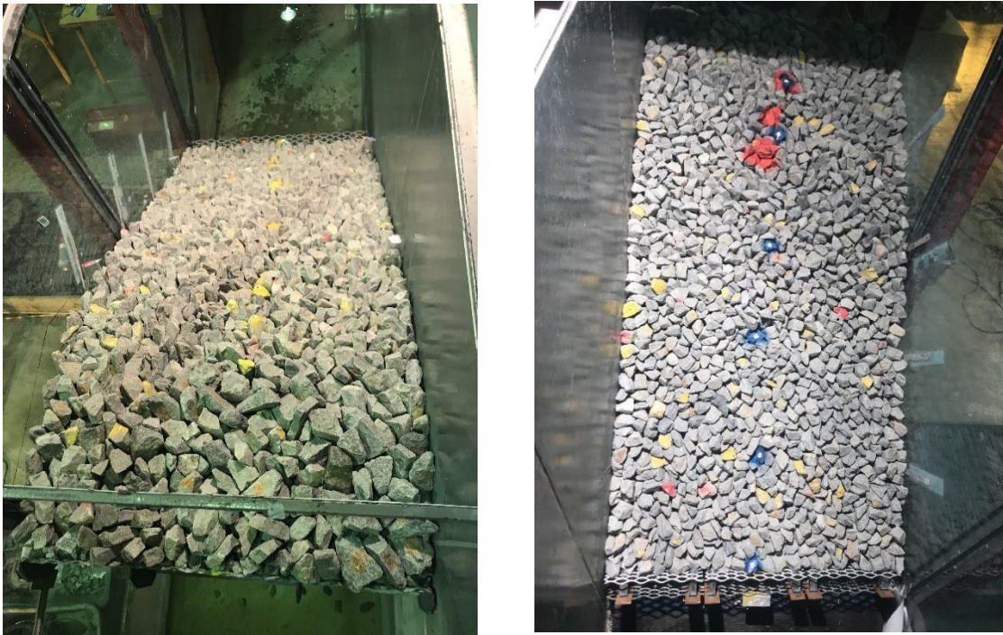
Figure 11 Constructed riprap ready for overtopping test with marked stones at specified distance from the toe for observing displacements. View from both upstream and downstream. View from downstream also shows installed load cells. Photos by K.N. Opere.
