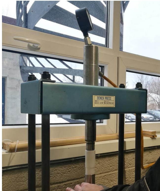
Figure 3.6: Compressing the soil sample using a bench press. Photo: Runa A. Solberg.
