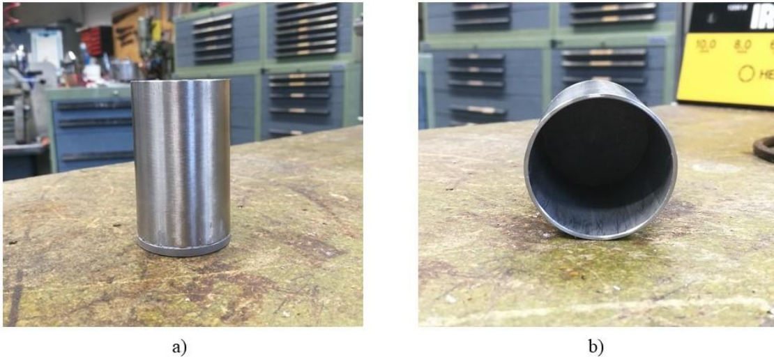
Figure 3.4: Second modification. a) cylinder and glued bottom filter and b) cross-section of cylinder with no soil sample inside. Photo: Runa A. Solberg.
