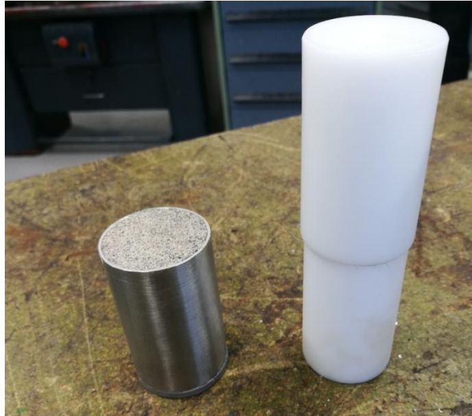
Figure 3.5: Packed sand sample in cylinder and POM rod. Photo: Runa A. Solberg.
