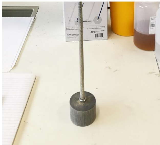
Figure 3.8: Rod used to compact sand samples in the modified Darcy-cell setup. Photo: Runa A. Solberg.
