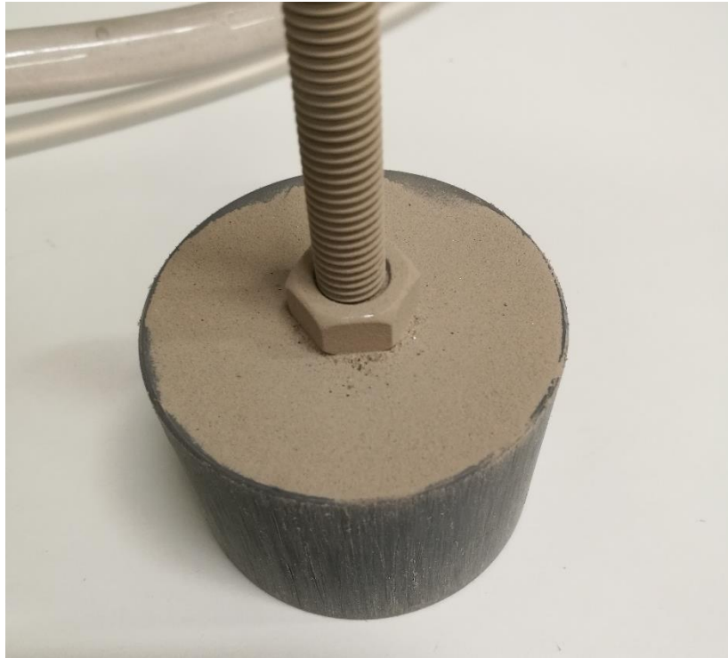
Figure 3.25: Fine material that has collected on the packing rod during the packing process in the Darcy-cell method. Photo: Runa A. Solberg.
