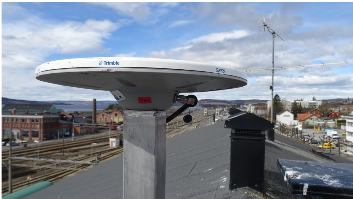
Figure 2.5: A permanent CPOS base station[15]
