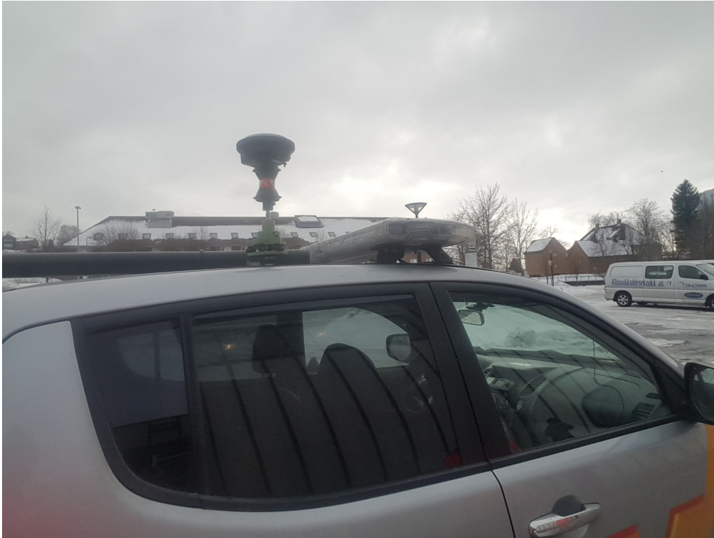
Figure 3.3: GNSS Receiver mounted on the prism, mounted on the roof of vehicle
