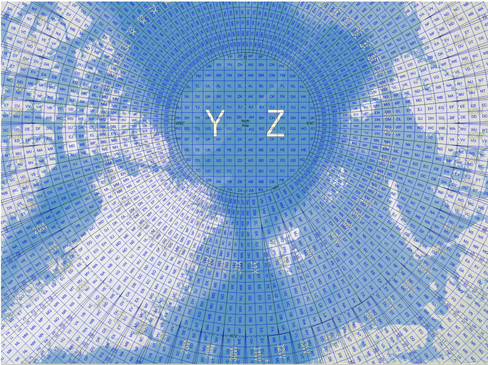
Figure 4.18: Illustration of the Military Grid Reference System, the geocoordinate standard used by NATO militaries for locating points on the earth. The 100km grid cells coincide with the Sentinel-2 images geographical footprints [51].
