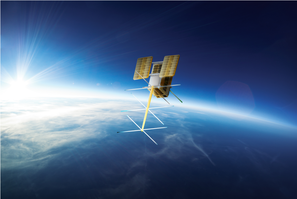
Figure 3.1: The Norwegian made satellite NorSat-2 launched July 2017. Among other equipment is an AIS transceiver [22].
