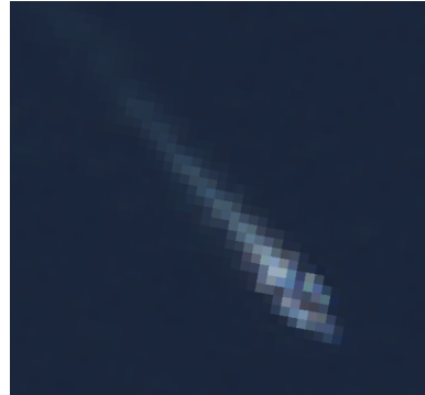
Figure 3.7: Ship found in Sentinel-2 TCI. Based on the pixel resolution of 10 m, we can estimate the length of the ship to be approximately 80 meters. This is only an approximation as it is hard to distinguish ship and wake only by observation.
