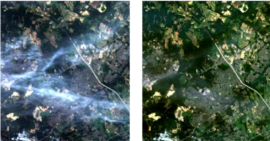
Figure 2.10: Level-1C TOA product (left) and corresponding Level-2A BOA product (right) generated by the Sentinel-2 Toolbox [16].
