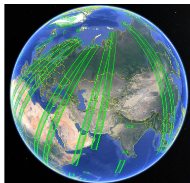
Figure 4.8: Visualisation of a priori acquisition plans for datatakes captured by the two Sentinel-2 satellites. The plans are for a time interval of 24 hours.
