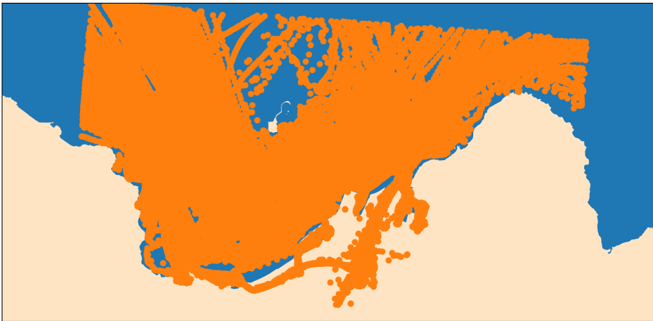
Figure 4.17: Visualisation of accumulated ship positions (orange dots) for 20 days, outside the port of Trondheim, Norway. 1.7 million AIS messages from 158 unique vessels, which is more than twice as many as the global count showed in Figure 4.16! A further note is that the restricted extent of the ship messages is due to the maximum receiving distance of the AIS shore receiver, not a result of the spatial or temporal filtering.
