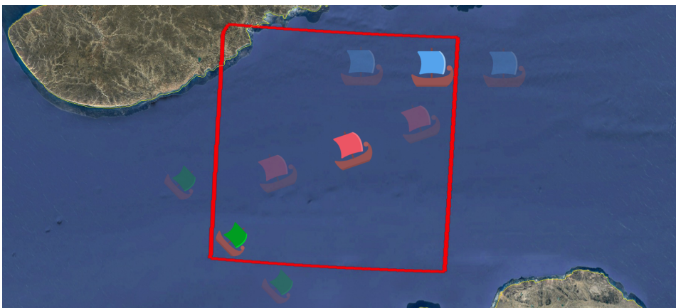
Figure 4.25: Illustration of different scenarios for interpolation of ship positions at the image timestamp. The transparent ships represent position each ship had when transmitting the AIS messages. The intermediate ships represent the ships position at the timestamp the image was sensed.
