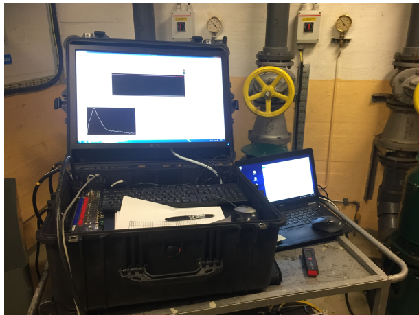
Figure 3.4: Set-up with computers for temperature and velocity measurements
