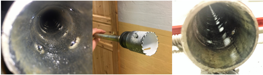
Figure 3.11: Measurement pipes before and after using the hole saw.
