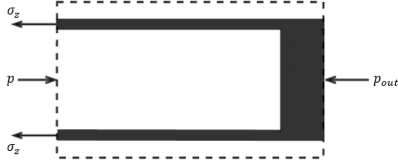
Figure 4.3.1: Free-body-diagram of a unrestrained, closed valve. The pressure force acts over an area A_f and the resulting axial stress acts over a area A_s [4].
