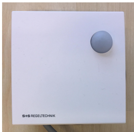
Figure A.4.: Sensor measuring light level.
