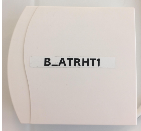
Figure A.5.: Sensor measuring the relative humidity.
