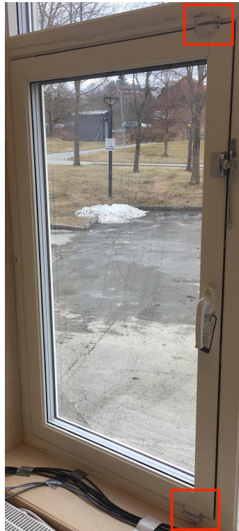
Figure 4.22.: Sensors registering window opening marked with the red boxes. Photo: Stina Skeie.
