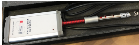
Figure A.7.: Anemometer measuring air velocity.
