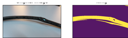
Figure 3.8: cv2.Treshhold on a broken cable
