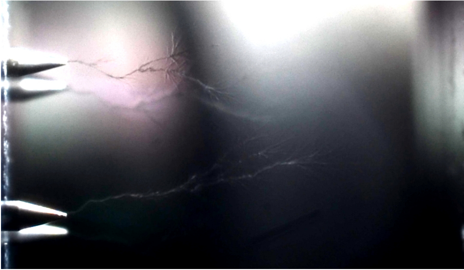
Figure C.3: SF 6 , positive needles at 2 mm
