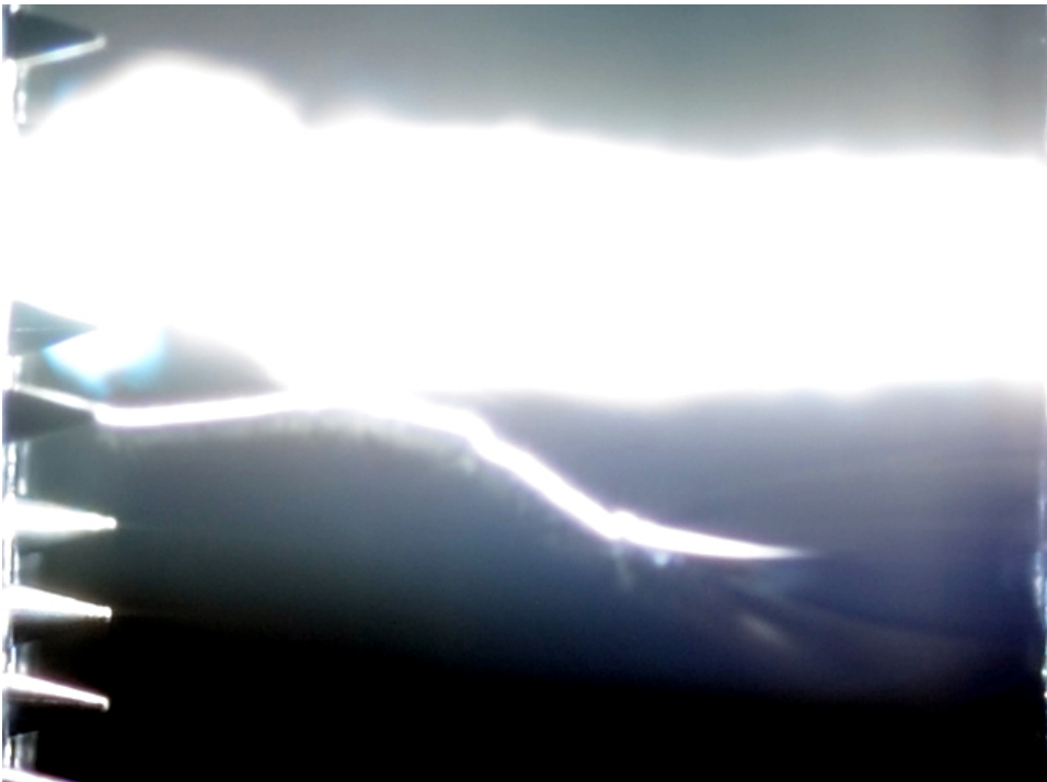
Figure C.6: SF 6 , negative needles at 1 mm
