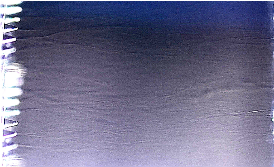
Figure 6.49: Heated channels at negative polarity in \text{CO}_2 with 100 needles at 0.5 mm length
