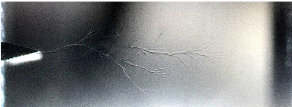
Figure C.4: SF 6 , positive needles at 2 mm
