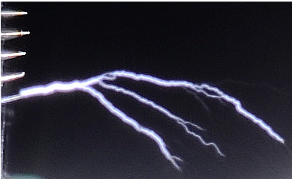
Figure 6.53: 20 needles at 0.5 mm and positive polarity in \text{CO}_2
