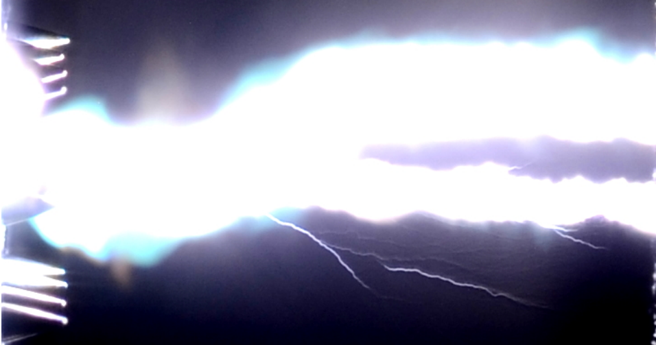
Figure C.15: CO 2 , positive needles at 1 mm
