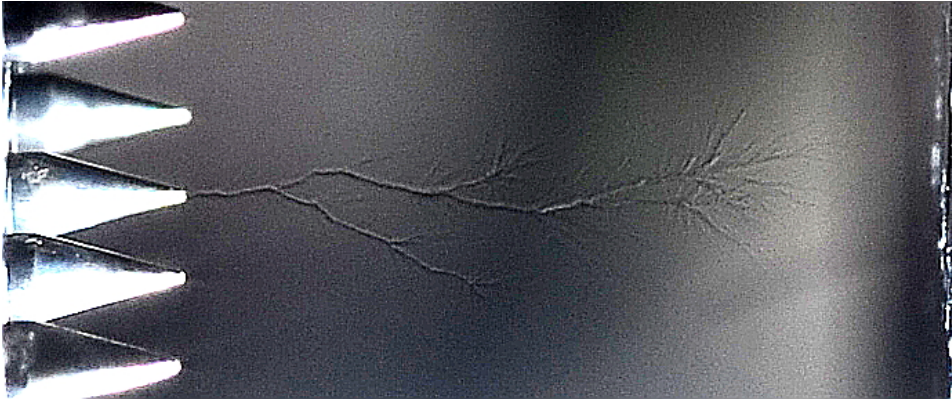
Figure C.7: SF 6 , positive needles at 2 mm
