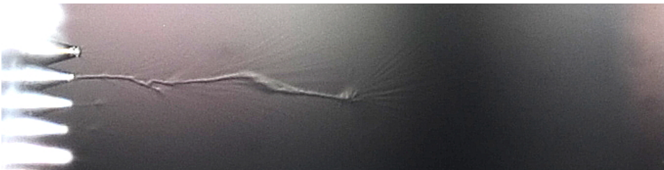
Figure C.9: SF 6 , negative needles at 0.75 mm
