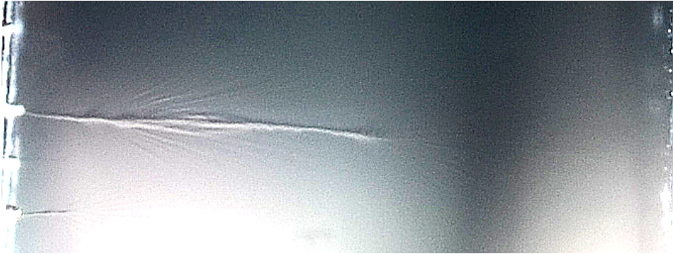
Figure C.5: SF 6 , negative needles at 0.2 mm
