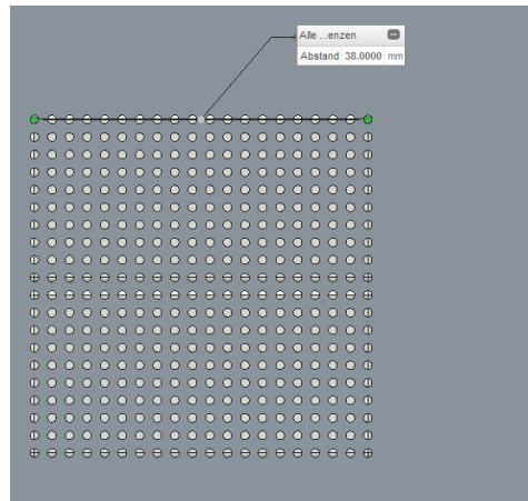
Figure 4.4: Top view of the design of the holes of the needle electrode.
