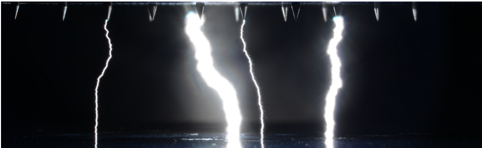
Figure 6.44: 16 needles at 2 mm and positive polarity in SF 6 .
