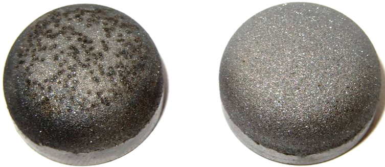
Figure 4.15: The actual plugs used, Plug A to the left after use and Plug B before use to the right.
