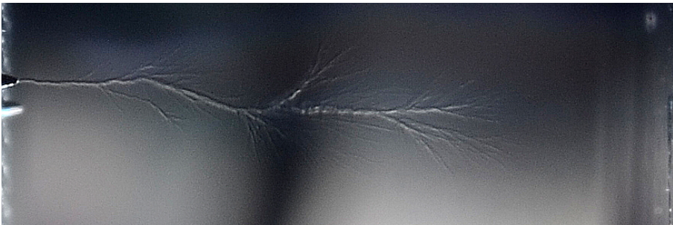
Figure C.2: SF 6 , positive needles at 0.5 mm
