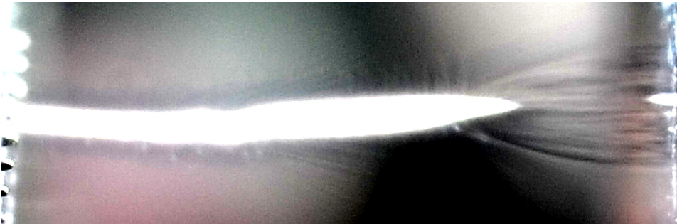
Figure C.8: SF 6 , negative needles at 0.2 mm
