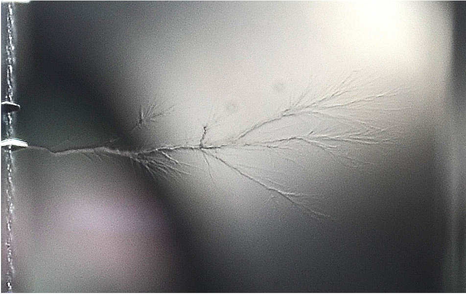
Figure 6.45: Positive leader channel with 0.5 mm needles in SF 6 . Enhanced with "sharpen effect" to better show the details.
