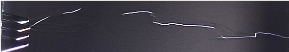
Figure 6.52: 20 needles at 1.0 mm and negative polarity in \text{CO}_2
