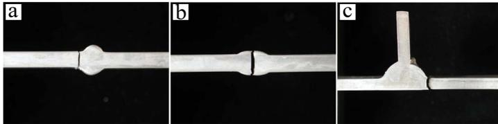
**Figure 5.1:** Failure points of the welded experimental specimens. (a) full penetration butt welded plate (crack initiation at weld toe), (b) non-penetrated butt welded plate (crack initiation at weld root), (c) transverse stiffener (crack initiation at weld toe). Image courtesy of Özler Karakaş [35]
