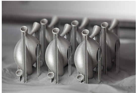
Figure 4: Left: Schematic illustration of powder bed fusion. Right: Picture of parts produced by selective laser melting [10].
