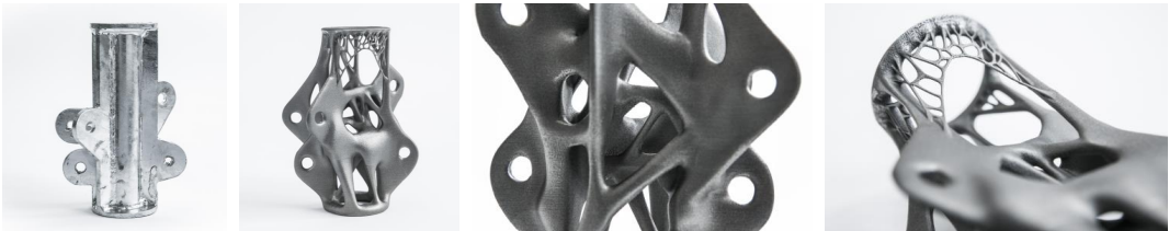
Figure 8: Topology optimised structure by S. Galjaard et al. [13]
