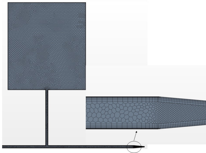
Figure 4.7: Representation of mesh for the outlet and one of the two accumulators.
