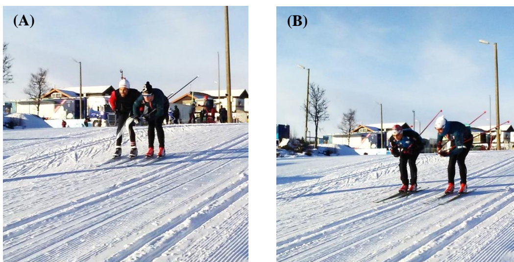
Figure 20: Parallel test by two Olympiatoppen technicians at the Norwegian National opening FIS competition at Beitostølen in November 2017. (A) The skiers are holding hands to equalize velocity. (B) The skiers run down the slope separately in a squat position
