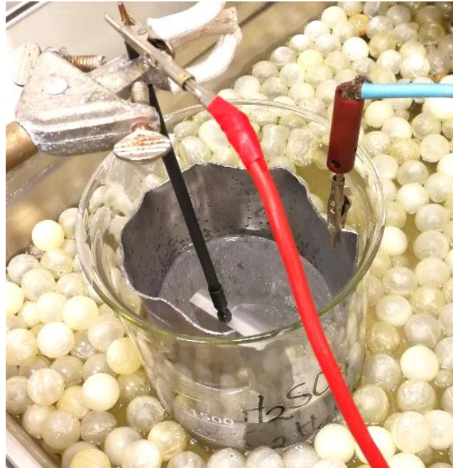
Figure 34: Setup for anodizing of aluminum
