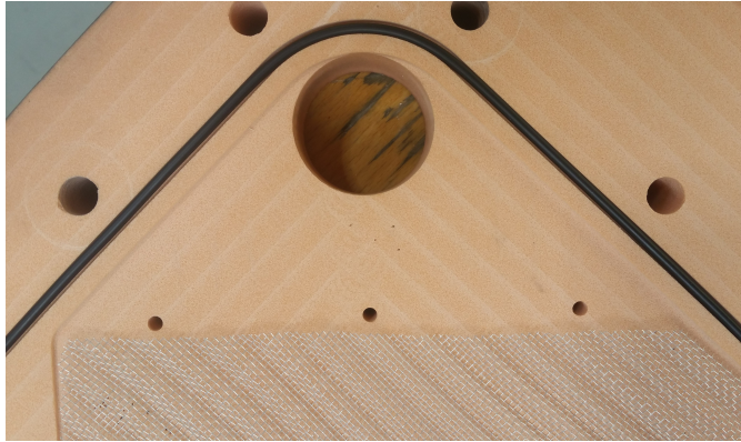
Figure 5.8: Pressure taps located before the effective exchanger area
