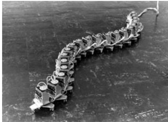
Figure 1.1: The Active Cord Mechanism model ACM III , the world's first robotic snake to achieve serpentine movements [4], in 1972.
