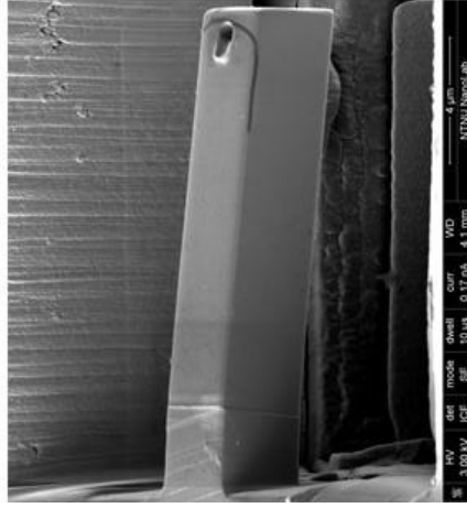
Cantilever 1: After bending (Air)
