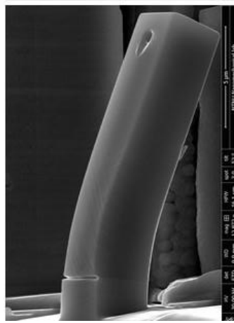
Cantilever 5: After bending (Air)
