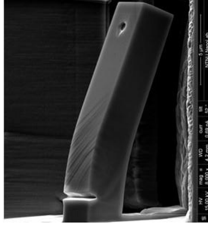
Cantilever 8: After bending (Air)
