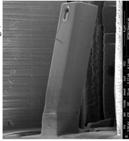
Cantilever 2: After bending (In-situ, 1 hour of H charging)
