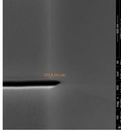
Cantilever 3: After bending (In air, 17 hours after H charge)
