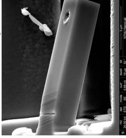
Cantilever 3: After bending (Air)
