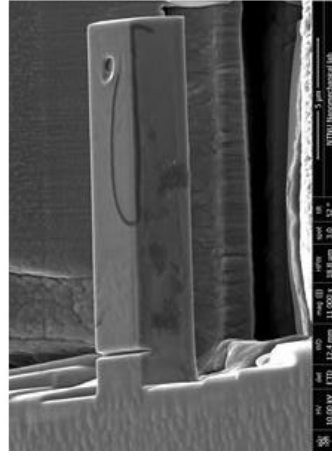
Cantilever 4: After bending (In-situ, 2 hours of H charging)
