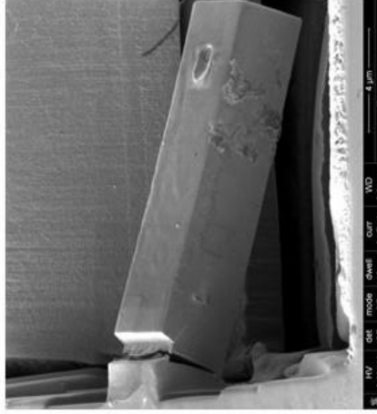
Cantilever 3: After bending (In air, 17 hours after H charge)
