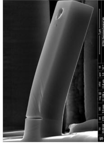
Cantilever 3: After bending (Air)
