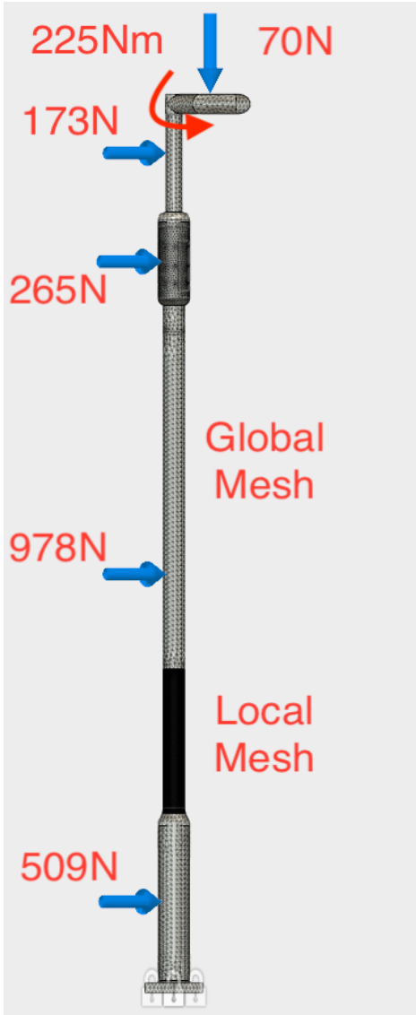
Figure 9.11: Simulation model with corresponding loads
