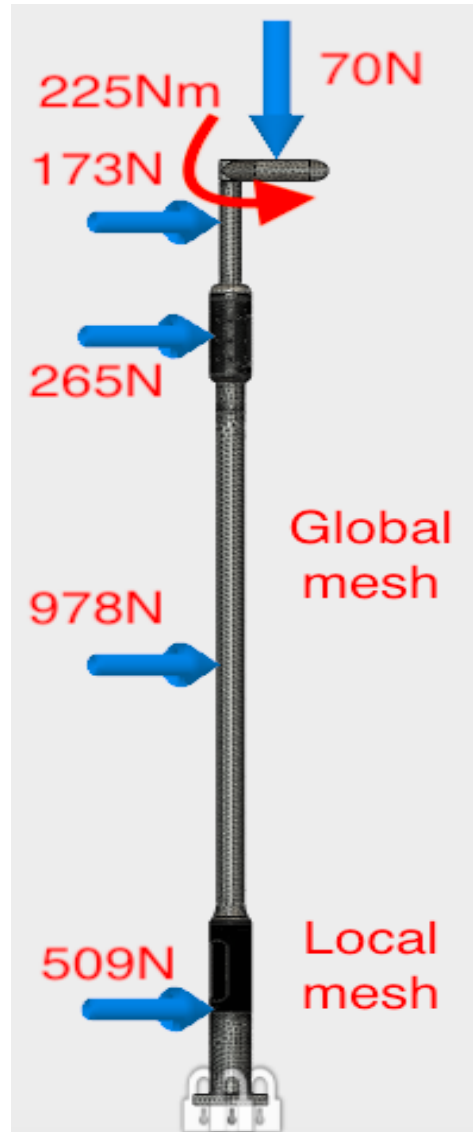
Figure 9.12: Simulation model with cut in bottom section
