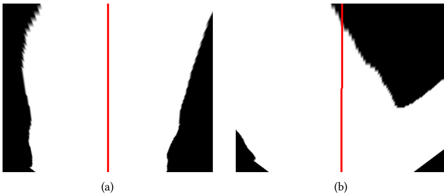
Figure 4.7: Two samples from the test set to visualize the path verification. (a) was a sample that passed the verification, while (b) did not. An error in the test set causes the all steering angles to be close to 0 degrees.
