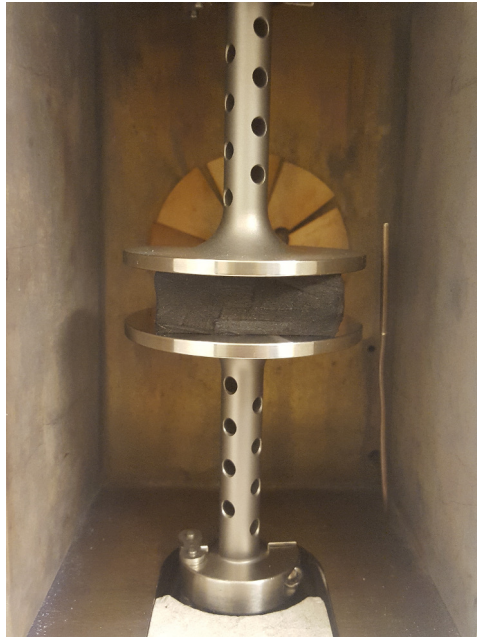
(a) Compressed test specimen.
