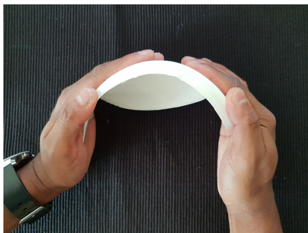
(c) Flexibility of ninjaflex insole.
