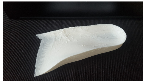
(b) NinjaFlex, Shore hardness: 85A.
