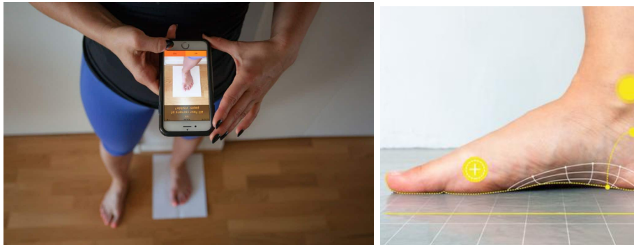
(a) 3D scanning of foot with the Wiiiv App. (b) Map each of the feet to over 200 data points.
