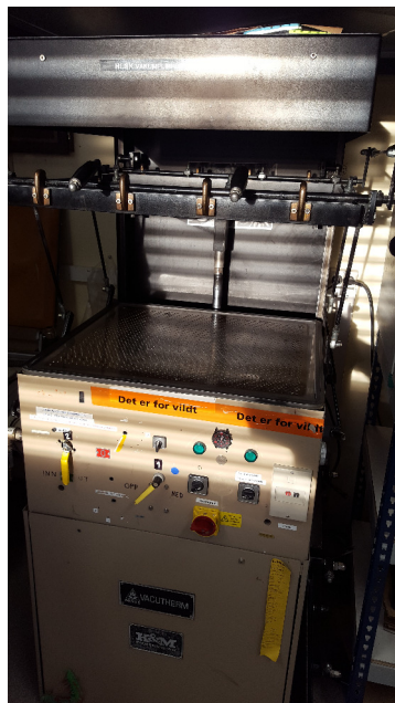
Figure 3.4: The vacuum forming machine used at TOV.
