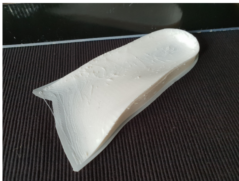
(a) Cheetah, Shore hardness: 95A.
