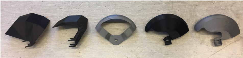
Figure 3.23: Five of the ten 3D-printed mudguards
