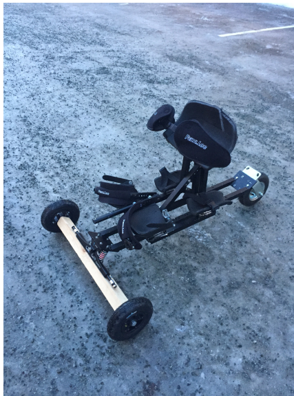
Figure 3.19: Three wheeled set-up with the axle length prototype
