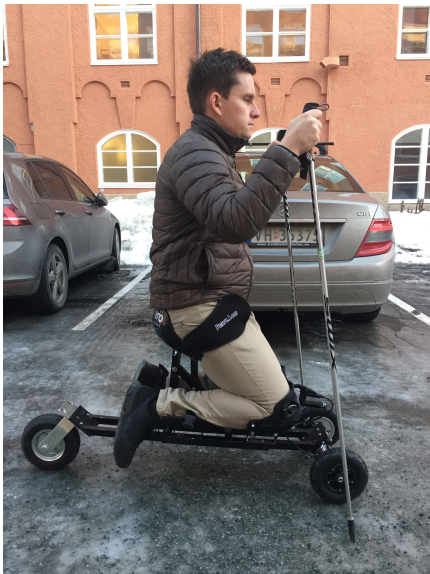
(a) Cobbled up wheelbarrow wheel mounted to Spike
