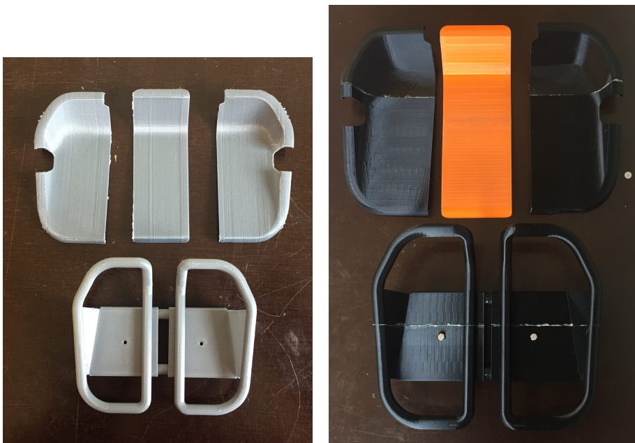
(a) Disassembled 3D-printed seat in 1:5 scale (b) Disassembled 3D-printed seat in 1:1 scale
