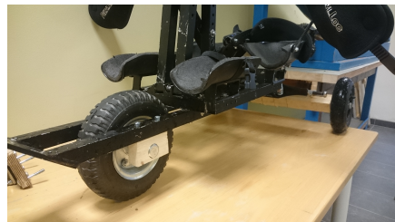
(b) Adjustable single wheel prototype mounted to Spike
