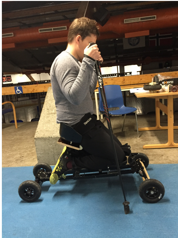
Figure 4.1: Normal truck back and increased axle length in the front
