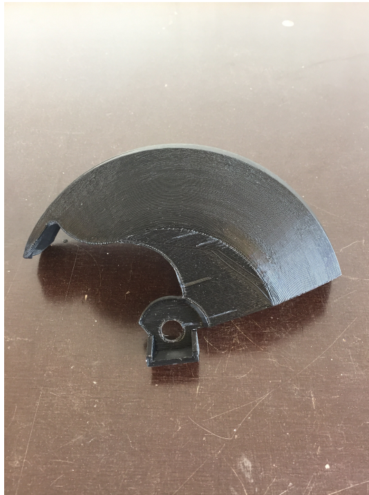
Figure 3.24: The final 3D-printed mudguard
