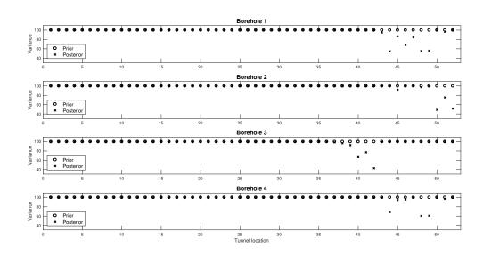
Figure 7: Variance reduction obtained by data in single boreholes 1, 2, 3 and 4.
