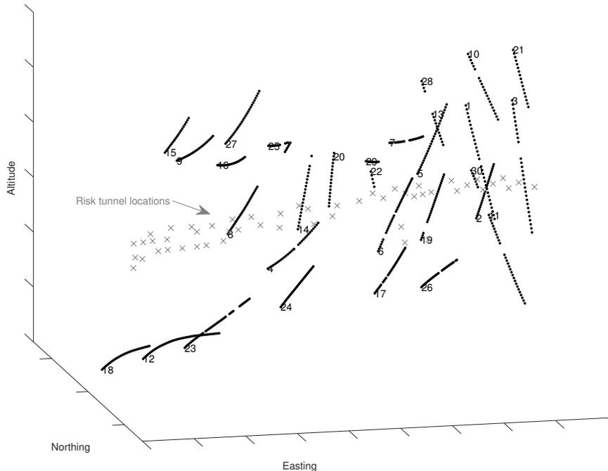
Figure 6: Risk tunnel locations and borehole design of 30 boreholes for joint frequency data.
