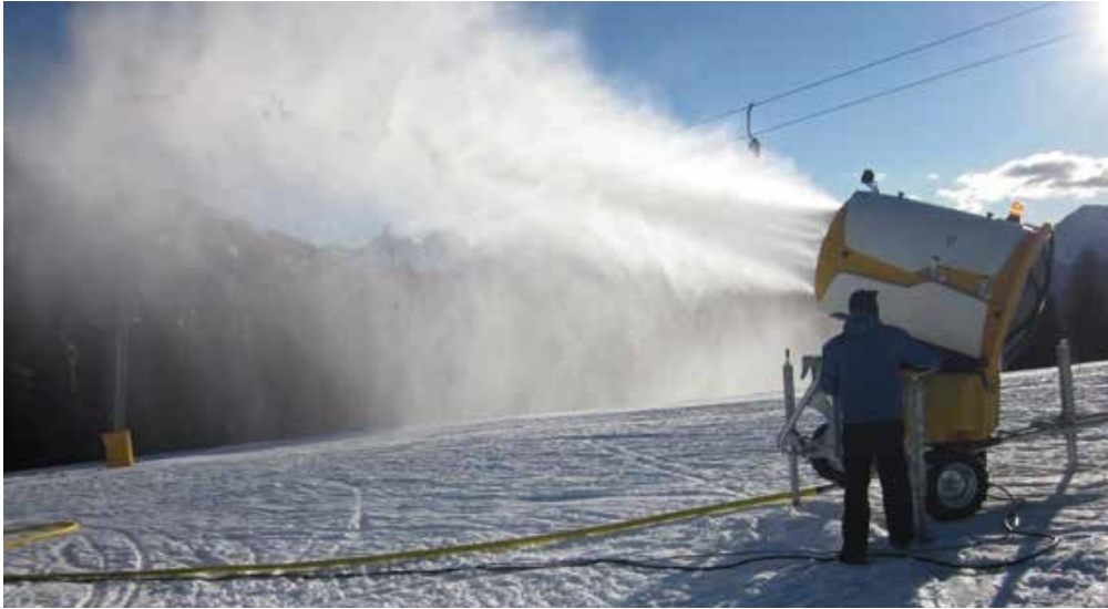
Figure 3.2: A mobile fan gun unit (Gjerland and Olsen, 2014)
