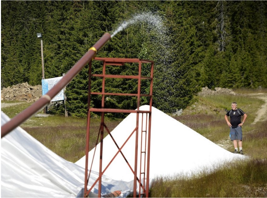
Figure 3.6: TIS production by a flake ice machine (SF220) at Sjusjøen, Norway (Müller, 2015)
