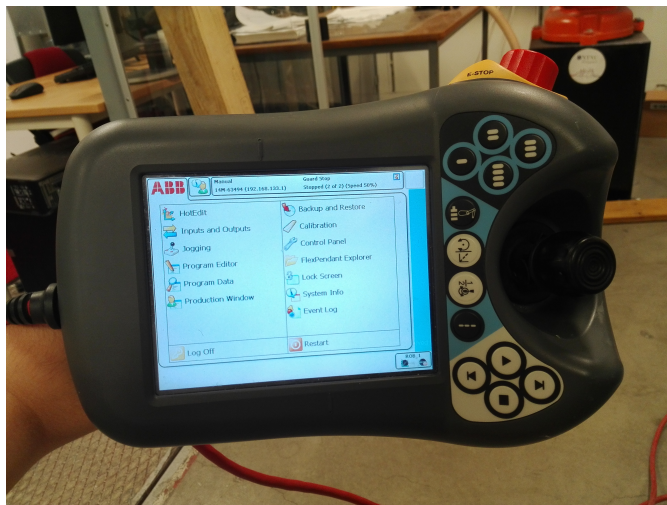
Figure 4.14: Window with main menu of FlexPendant at laboratory
