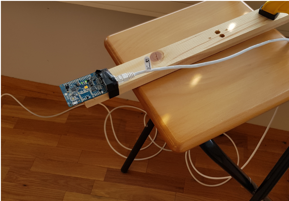
Figure 5.3: Test setup RSSI - distance relationship. The node is elevated 75cm. The tag is set up in the same way, both with antennas in free air, and free line of sight.
