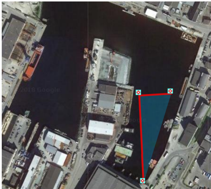
Figure 2.6: Triangle for Calculating x,y position of boat from lat-lon coordinates
