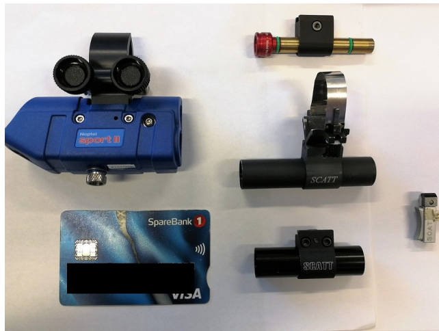
Figure 2.4: Overview of Noptel Sport II and SCATT systems [5]. Left side: Noptel Sport II unit and debit card for reference. Middle column from the top: SCATT WS-M02(IR), SCATT Biathlon (IR), SCATT USB (Wired). Right side: SCATT trigger measurement unit.
