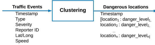
Figure 24: The input and output of the clustering module.
