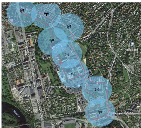
Figure 7: A hypothetical situation where the path from figure 6 is entirely covered by RSUs, shown as antennas. Their receptive fields are shown as blue circles. The figure is from [1].
