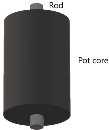
Figure 5.12: Illustration of the revolved 2D-axisymmetric FEM model
