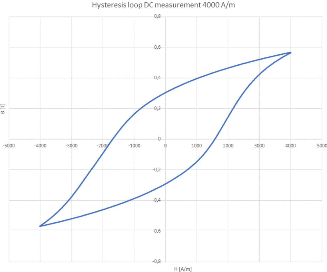
Figure 5.4: Measured DC hysteresis loop in material 2 at 4000 A/m
