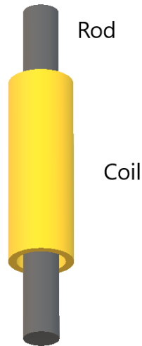
Figure 5.11: Illustration of the revolved rod and coil in the 2D-axisymmetric FEM model
